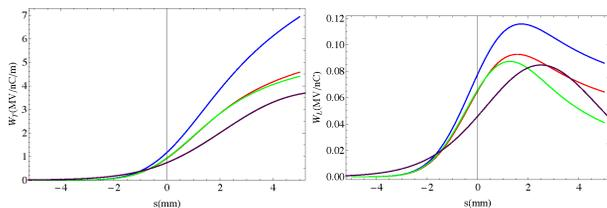
Figure 3: Comparison of wake potentials. Right and left figures show transverse and longitudinal wake function, respectively. Green, red, blue, and purple lines show K. Yokoya, K. Bane, analytical, and calculated wake function (CST), respectively.
