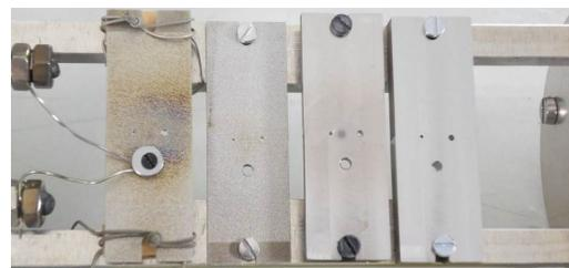
Figure 4: Photo of the targets after irradiation.
