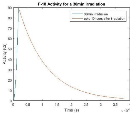
Figure 6: Activity of F-18 obtainable using QGSP\_BIC\_AllHP.
