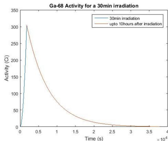
Figure 4: Activity of Ga-68 obtainable using QGSP\_BIC\_AllHP
