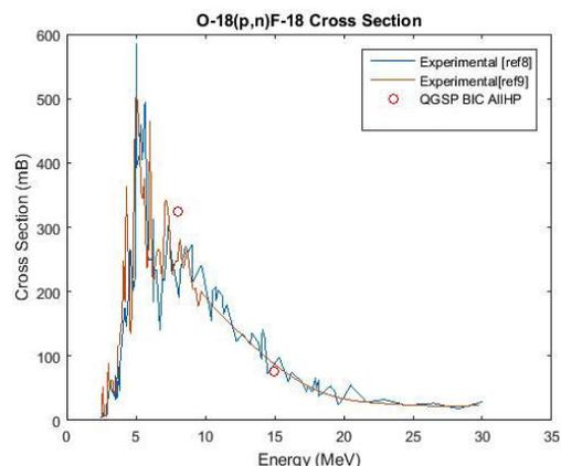
Figure 2: Experimental and simulated cross section results for the production of F-18 [7, 8].
