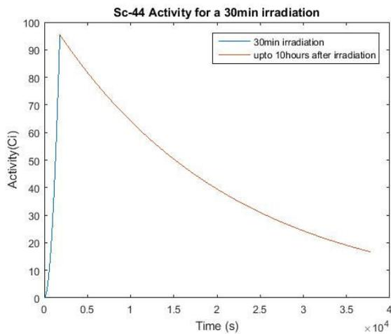
Figure 7: Activity of Sc-44 obtainable using QGSP\_BIC\_AllHP
