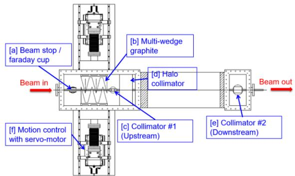
Figure 3: Schematic view of the multi-wedge degrader.
