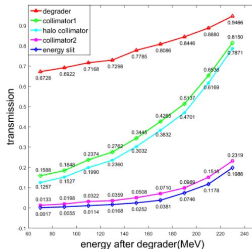
Figure 5: Transmission for energy degrading to 70-230MeV.
