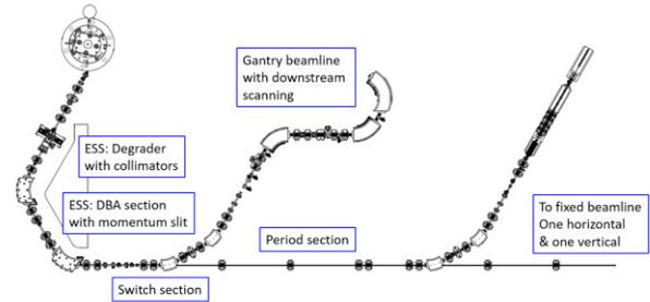
Figure 1: Layout of the beamline.
