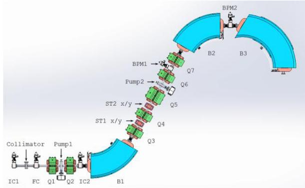
Figure 7: Layout of the gantry beamline with downstream scanning (Scanning magnets and nozzle not shown).
