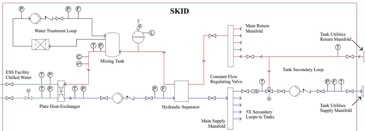
Figure 3: Functional scheme of the SKID proposed.
