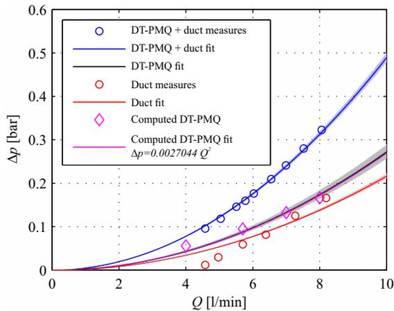
Figure 2: Experimental measures, CFD simulations and corresponding best fits.
