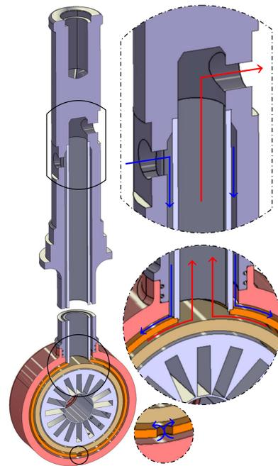
Figure 1: Internal layout of a DT-PMQ with water distribution.
