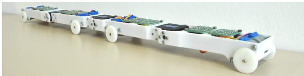
Figure 4: 3D printed prototype of the inspection robot.
