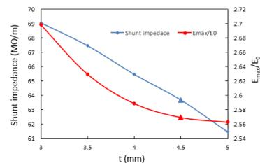
Figure 1: The shunt impedance and  $E_{max}/E_0$  VS. disk thickness  $t$ .
