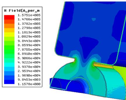
Figure 10: The peak magnetic field at the coupler windows.
