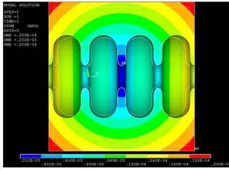
Figure 3: The deformation caused by temperature variation.
