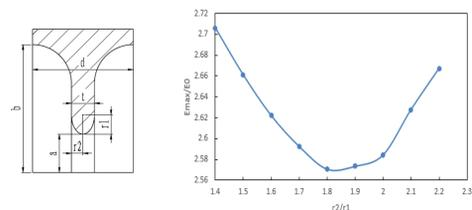
Figure 2:  $E_{max}/E_0$  as a function of the iris ellipticity.
