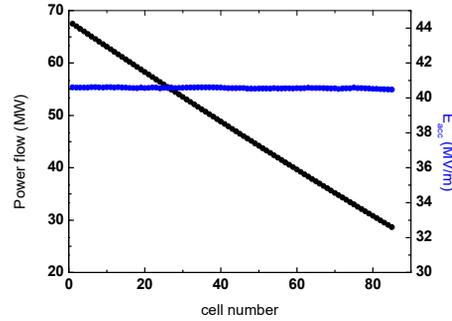
Figure 6: The power flow and  $E_{acc}$  along the structure.
