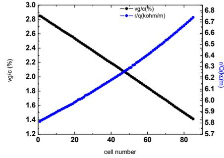
Figure 5: Each cavity's  $v_g$  and  $r/Q$ .
