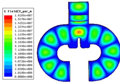
Figure 8: The electromagnetic distribution of the splitter.
