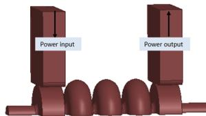
Figure 9 (a): The simulation model of the coupler.
