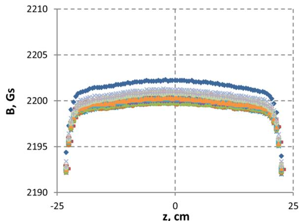
Figure 3: Field profile of a BM3 magnet near the magnet centre. Data from 16 Hall probes at different horizontal (x) positions ( $-7.5 \text{ cm} < x < 7.5 \text{ cm}$  with  $\Delta x = 1 \text{ cm}$ ) are shown.
