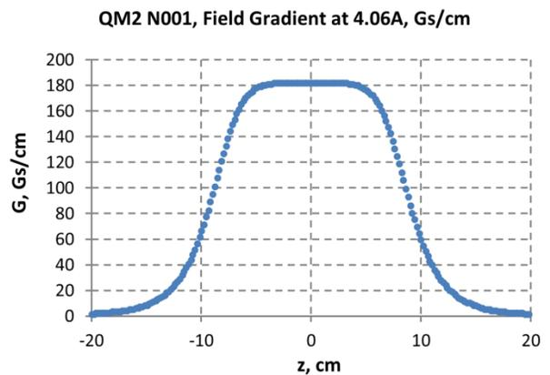
Figure 2: Gradient profile of a QM2 magnet derived from the Hall probe measurement. z is the coordinate along the beam axis.
