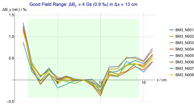
Figure 4: Homogeneity of magnetic field in the centre (z) of 8 BM3 magnets, measured with 16 Hall probes. The field is normalised to the central (x = 8 cm) Hall probe. Good field region ( $\Delta B = 4$  Gs,  $\Delta x = 13$  cm, shown as green rectangle) is within specification. Probe to probe systematic error of  $\sim 0.3\%$  can be seen.
