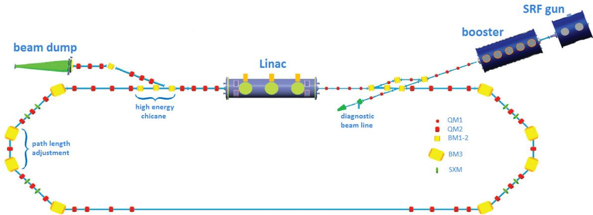
Figure 1: Layout of the bERLinPro magnetic system.
