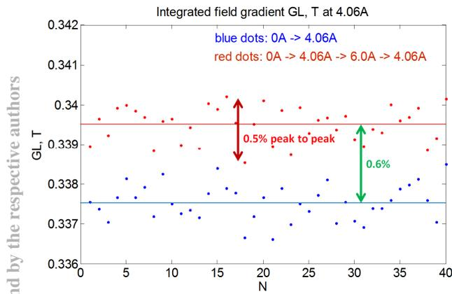
Figure 6: Integrated gradient of 40 QM2 quadrupoles measured with the rotating coil. The measurement allows estimating the spread of the quads strength and importance of the special turn-on procedure, which is chosen as increasing the current to 6.0 A and reaching the set value afterwards from above.
