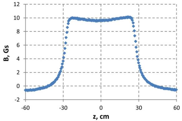
Figure 7: Residual field profile of a BM3 magnet. The central Hall probe is used.
