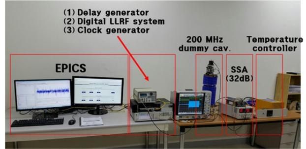
Figure 5: Test bench of digital LLRF system.
