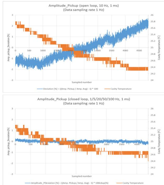
Figure 6: Comparison open loop and closed loop. (Upper) open loop test, (lower) closed loop test.
