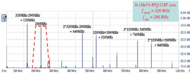
Figure 3: DAC output spectrum without BPF.
