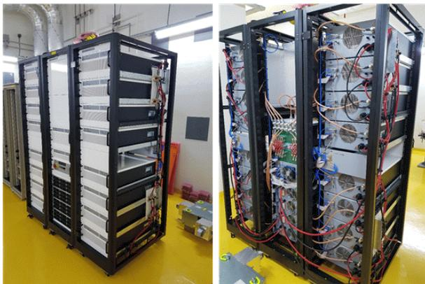
Figure 7: 240 kW SSA. (Upper) block diagram, (lower) picture of SSA located in KOMAC building.
