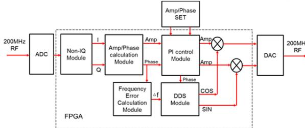
Figure 4: User FPGA controls logics.
