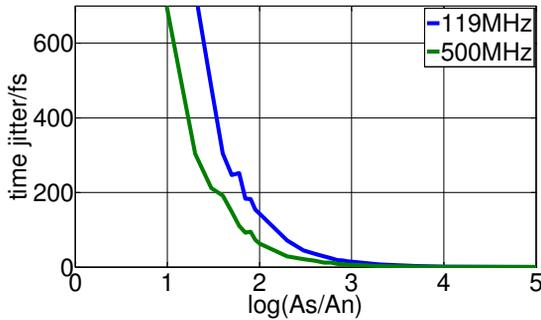
Figure 4: Time jitter in different SNR and sampling rate.
