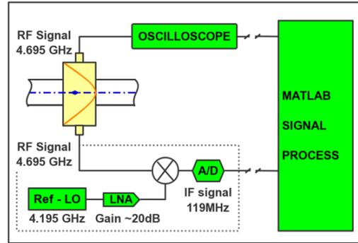
Figure 5: Signal process schematic diagram
