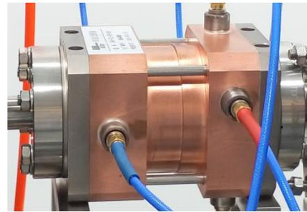
Figure 2: Prototype of CBPMs at DCLS
