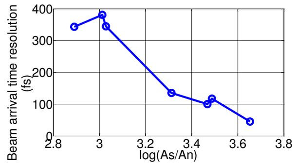
Figure 10: Beam arrival time resolution in different SNR
