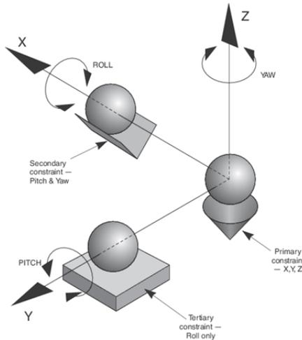
Figure 2: Simplified kinematic connection theory ©@ Newport Corp. [5].
