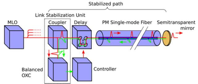
Figure 1: Simplified link stabilization scheme.
