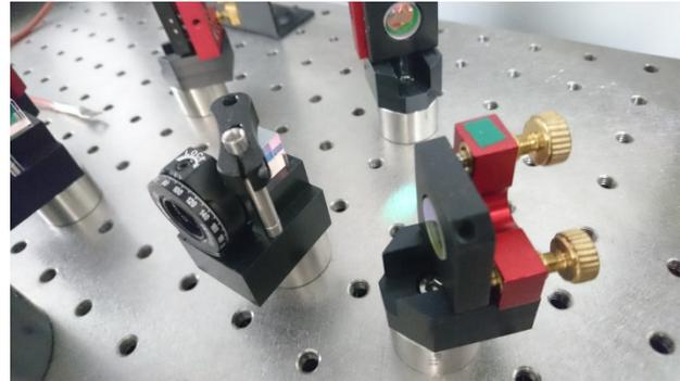
Figure 4: Mirror mount and beam splitter in the FSD of the XFEL synchronization laboratory.
