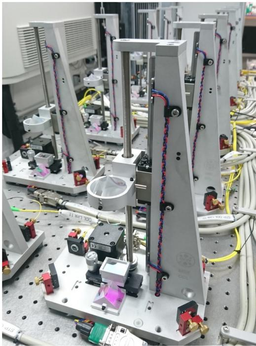
Figure 6: Optical delay lines on secondary steel table.
