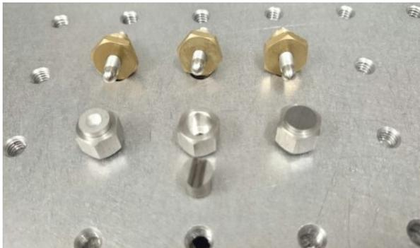
Figure 3: Kinematic mounting supports for larger devices.
