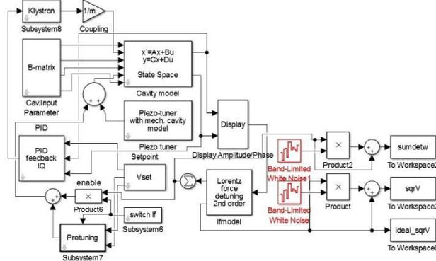
Figure 2: Cavity state-space model equipped with phase and amplitude noisy sources.
