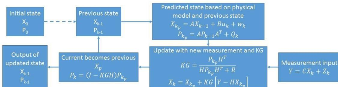
Figure 1: The multi-dimension model of Kalman filter based on matrix arithmetic.
