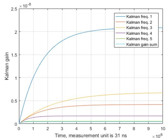
Figure 4: KG stabilises after some time depending on initial noise matrixes choice.
