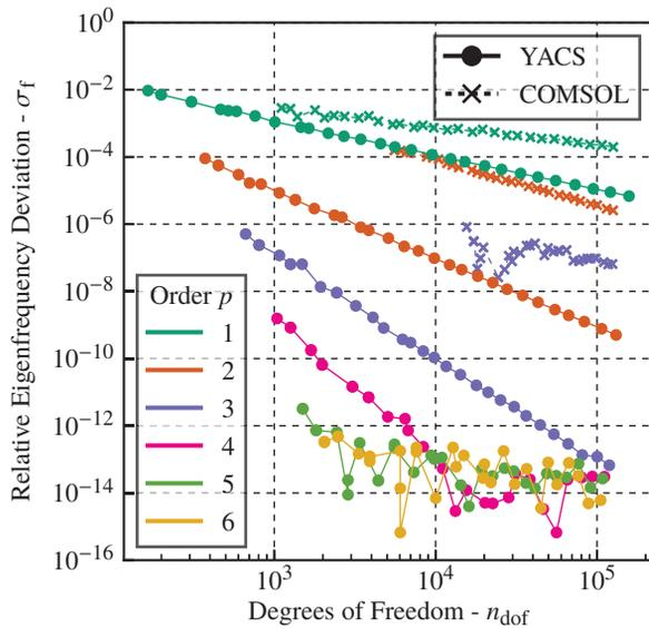
Figure 2: Relative eigenfrequency deviation  $\sigma_f$  of the first dipole mode of a pillbox resonator, obtained from YACS and COMSOL (3D) as a function of the number of degrees of freedom  $n_{dof}$  for different polynomial orders  $p$  of the function basis. The frequency deviations were calculated with respect to the analytical solution.
