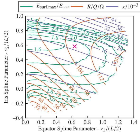
Figure 3: Parameter space scan for the subset of spline parameters within the non-reentrant regime of cubic spline cavities. Displayed are the figures of merit  $E_{surf,max}/E_{acc}$ ,  $R/Q$  and the coupling constant  $\kappa$  for the  $TM_{010,\pi}$ -Mode. The red cross represents the final cubic spline parameters for the optimization of the cost function (see Fig. 4).
