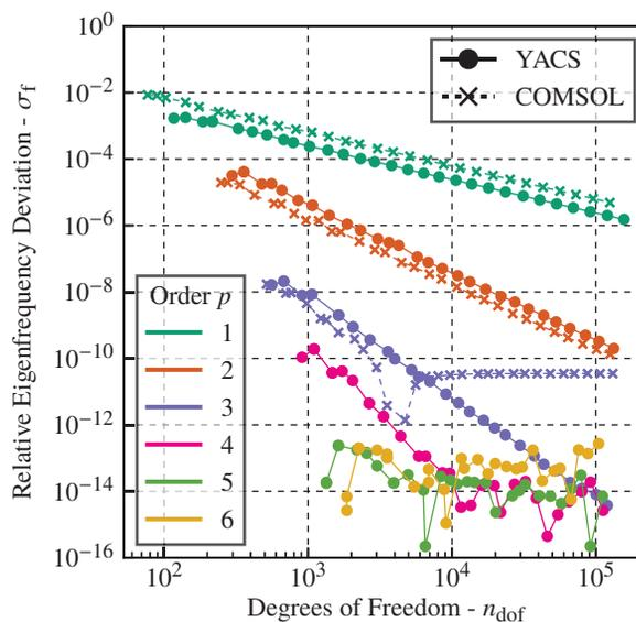
Figure 1: Relative eigenfrequency deviation  $\sigma_f$  of the first monopole mode of a pillbox resonator, obtained from YACS and COMSOL as a function of the number of degrees of freedom  $n_{\text{dof}}$  for different polynomial orders  $p$  of the function basis. The frequency deviations were calculated with respect to the analytical solution.
