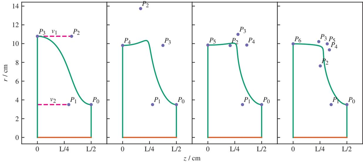
Figure 4: Optimized shapes and their respective control points for the different spline orders in ascending order. Each shape optimization for  $n > 4$  used the optimization result of the previous order as the initial guess, utilizing the degree elevation algorithm. In the case of cubic spline cavities the parameters  $v_1$  and  $v_2$  represent the only degrees of freedom of the curve, since the r-coordinates are fixed due to the  $C^1$  continuity requirements [12].
