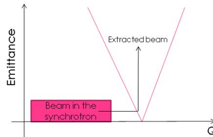
Figure 4: Steinbach diagram for extraction at CNAO: beam is driven into the resonance by a betatron core.
