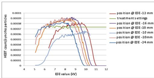
Figure 5: extraction efficiency (arbitrary units) as a function of beam position at ESE, and ESE strength.
