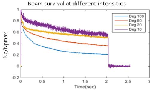
Figure 1: Beam current in the ring at different intensities: the current is normalized to its maximum value.
