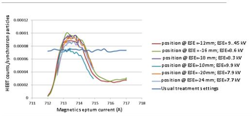
Figure 6: extraction efficiency (arbitrary units) as a function of beam position at ESE, and MSE strength.
