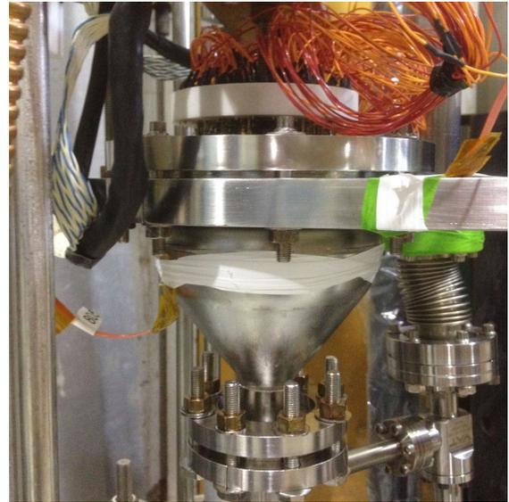
Figure 1: The Cornell sample host cavity, shown here installed on the test insert with the temperature-mapping system mounted on the sample plate, laying horizontally on the top of the cavity.
