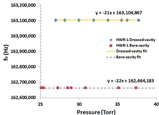
Figure 7: Frequency vs. LHe Pressure when the bare cavity was cooled from 4.2K to 2K.
