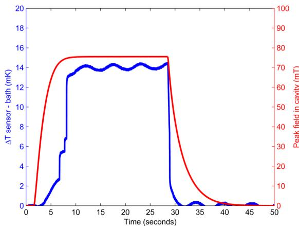
Figure 3: A single-scan trace, showing the RF field in the cavity (in red) and the temperature of the sensor at located at the quench origin (in blue). The oscillations seen on the temperature signal are due to the valve oscillations from the pumping system that keeps the bath temperature at 2.0 K.
