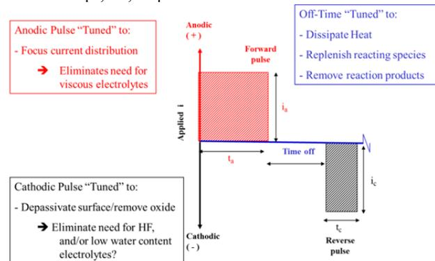
Figure 4: General bipolar EP process representation [8].
