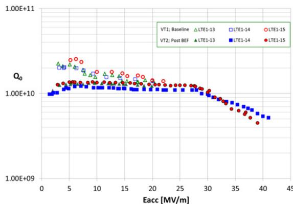
Figure 6: RF test results from the 1<sup>st</sup> and 2<sup>nd</sup> RF test runs at 2K.
