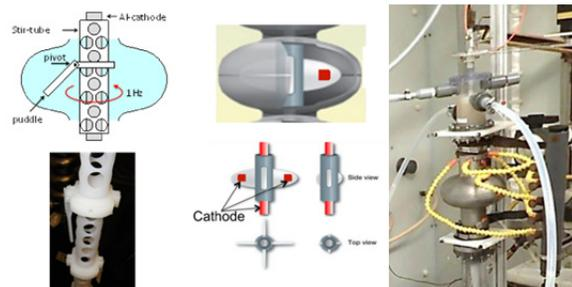
Figure 1: Images of Cornell VEP cathode (left); Marui's i-cathode Ninja type-I (middle), and single cell on the VEP stand at Cornell.
