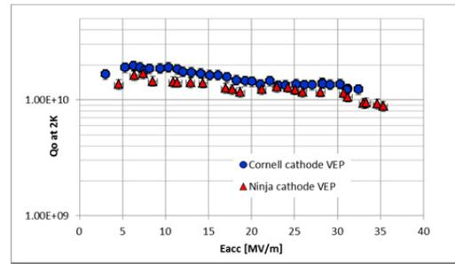
Figure 3: RF test results of NR1-2 at 2K.
