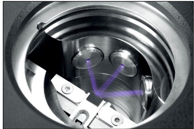
Figure 1: Leica TIC 3x sample chamber with triple argon ion beams. Sample location is at beam convergence point.
