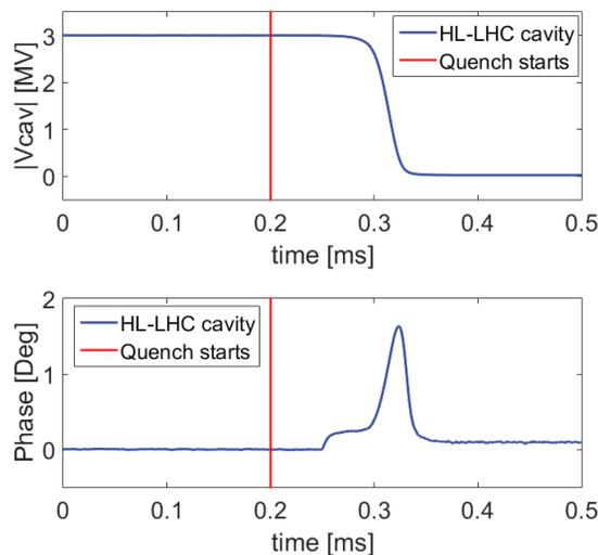
Figure 3: Magnitude (top) and phase (bottom) of the voltage for an HL-LHC-like crab cavity during a quench.
