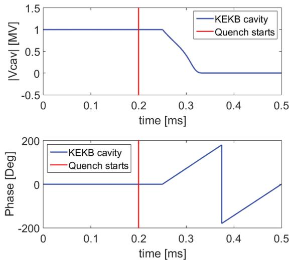
Figure 2: Magnitude (top) and phase (bottom) of the voltage for a KEKB-like crab cavity during a quench.
