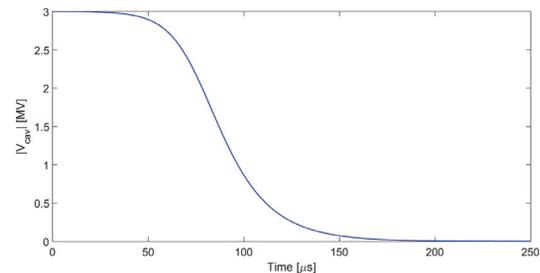
Figure 1: Magnitude of transverse voltage vs. time during a quench, neglecting all other effects.
