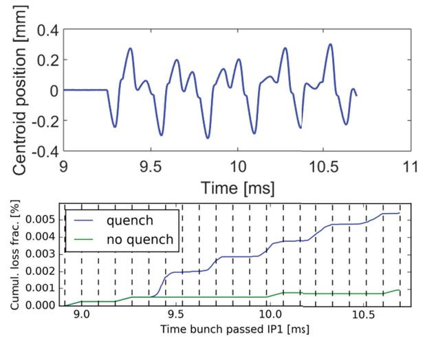
Figure 4: SixTrack simulation of a the mean beam position at the cavity (top) and the beam losses during a quench (bottom) of a HL-LHC-like crab cavity; vertical lines indicate turns.
