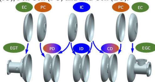
Figure 1: The cavity subcomponents.
