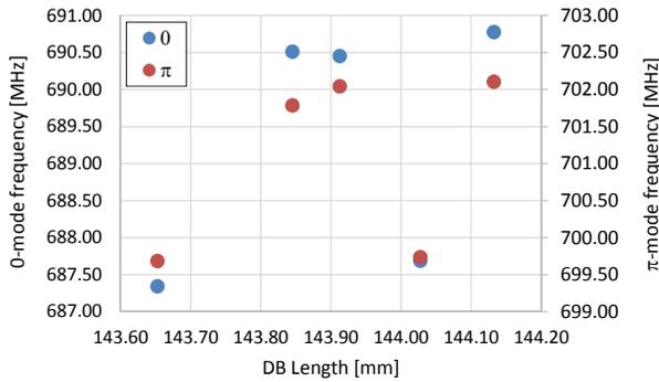
Figure 3: DB modes frequency spread after trimming.
