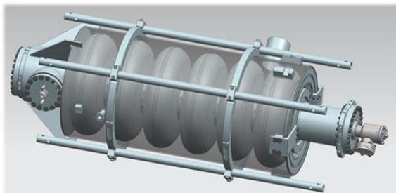
Figure 2: the “dressed” cavity (He-tank transparent to see the inner cells) equipped for the cold RF test.
