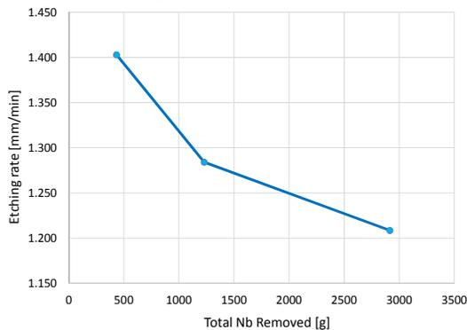
Figure 4: Etching rate versus total removed Niobium.
