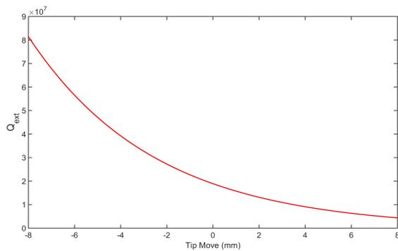
Figure 6: Change in  $Q_{\text{ext}}$  as the coupler penetration depth is increased and decreased.
