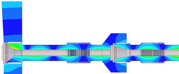
Figure 3: The magnetic field in the coupler for 16 kW input power.
