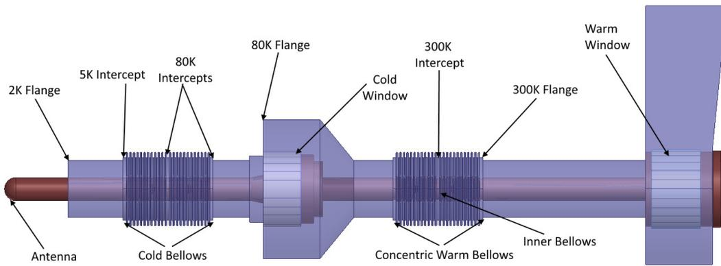
Figure 1: Basic RF design of the 1.5 GHz coupler showing only the vacuum and inner coupler. With temperature intercepts and components clearly labelled.
