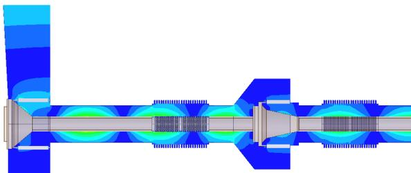
Figure 4: The electric field in the coupler for 16 kW input power.
