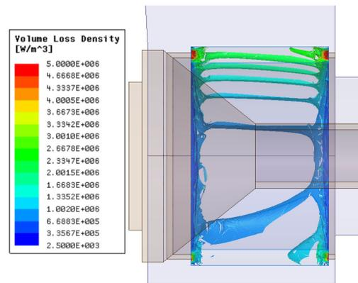
Figure 8: Volume loss density in the ceramic highlighting the point of high power loss that result in heating.
