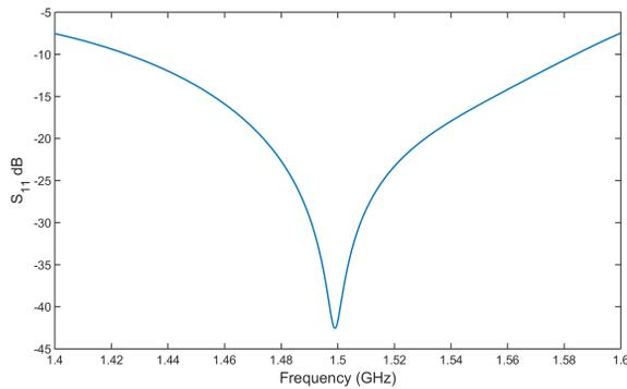
Figure 2: The  $S_{11}$  parameters for the final coupler design.
