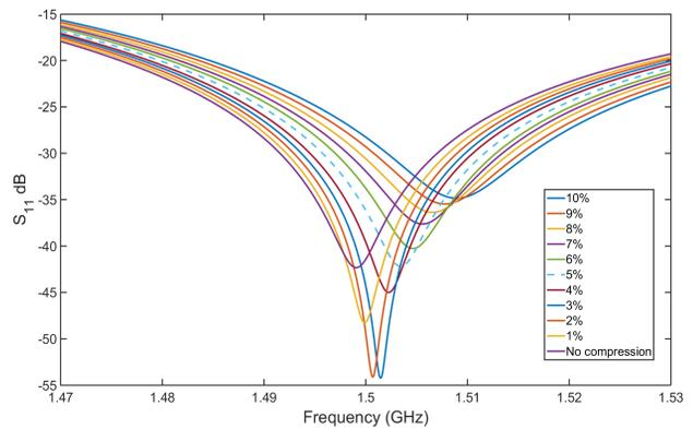
Figure 5: Change in  $S_{11}$  as the bellows are compressed by 10%.
