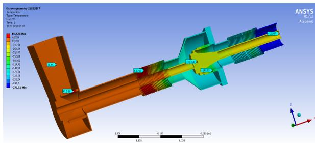
Figure 7: Thermal simulation for 16 kW travelling wave power.
