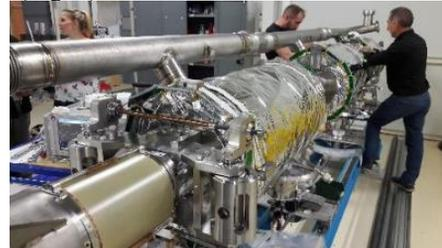
Figure 6: Piezo tuners assembly after the helium diphasic pipe in titanium has been welded.
