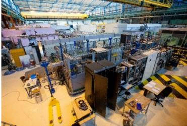
Figure 8: The RF 1.1 MW power source at 704MHz pulsed at 14 Hz, 3.6 ms used for the couplers RF processing and for the tests of the M-ECCTD.
