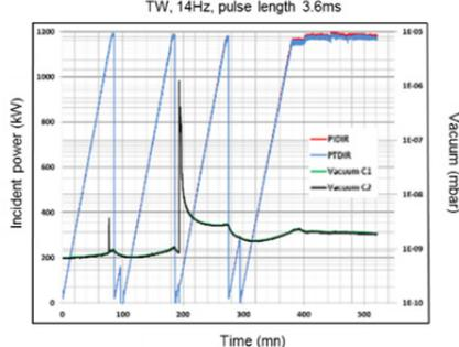
Figure 4: Vacuum pressure vs RF power during RF processing of a pair of power couplers in TW mode at 14Hz and the maximum pulse length of 3.6 ms.
