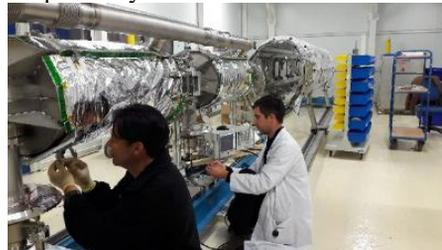
Figure 7: Last operations on the cavity string are in progress before insertion inside the thermal shield that has already been prepared (behind the cavity string).
