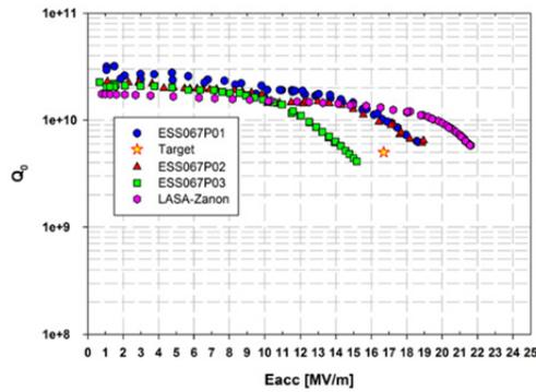
Figure 2: Q curves of the cavities mounted in the M-ECCTD.
