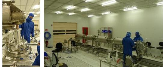
Figure 5: Assembling of the coupler on cavity (left) and of the cavity string (right) inside the ISO4 clean room.
