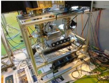
Figure 3: A pair of couplers mounted on a coupling box during the RF processing at room temperature.
