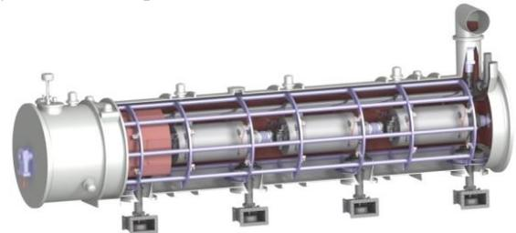
Figure 1: General layout of the ESS elliptical cavity cryomodule.
