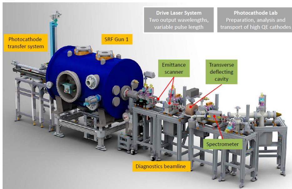
Figure 2: Gun1 cryomodule, photocathode transfer system, and GunLab diagnostics beamline.
