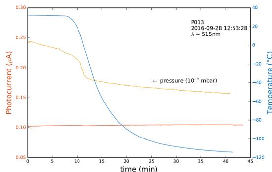
Figure 3: Data of photo-current measured at cathode P013 during cooldown from room temperature to  $-120\text{ }^\circ\text{C}$ . Shown are photocurrent, temperature and base pressure inside the growth chamber.
