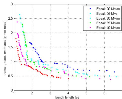
Figure 1: Pareto-optimum curves from MOGA runs with Gun1 at five different peak electric RF field values.
