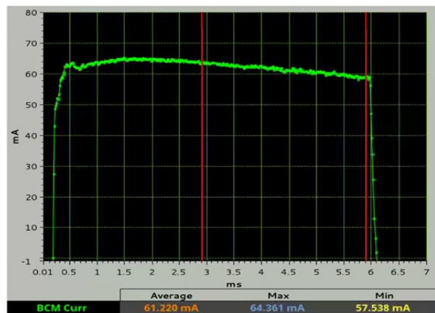
Figure 4: ACCT-measured pulse of the HVPS of the ESS ion source, courtesy of Lorenzo Neri (INFN-Catania) and Oystein Middtun (ESS).
