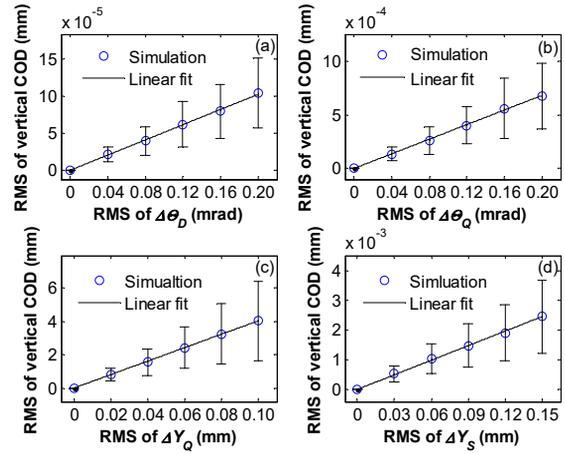
Figure 1: RMS of vertical COD resulting from (a) tilts of dipole, (b) tilts of quadrupoles, (c) vertical misalignments on quadrupole magnets and (d) vertical misalignments of the sextupole magnets.
