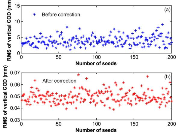
Figure 3: RMS of the vertical COD of 200 (a) uncorrected and (b) corrected random machine seeds.
