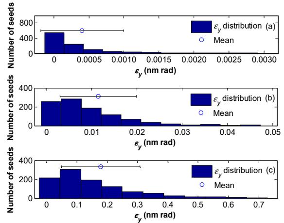
Figure 2: Distribution of vertical emittance from (a) tilts of dipole, (b) tilts of quadrupoles, (c) vertical misalignments of sextupole magnets for random seeds.
