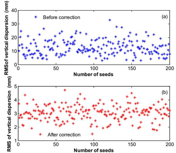
Figure 5: RMS of the vertical dispersion of 200 (a) uncorrected and (b) corrected random machine seeds.
