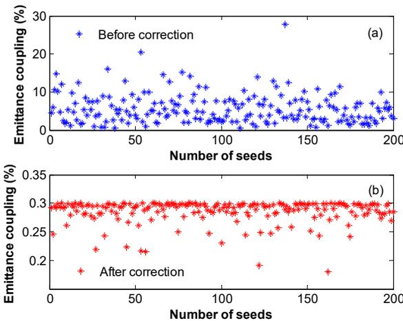
Figure 4: Emittance coupling of 200 (a) uncorrected and (b) corrected random machine seeds.
