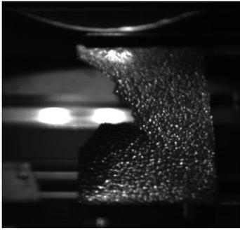
Figure 2: Image of a partially broken foil (Foil 4) as recorded by the BTV camera. The  $H^-$  beam was hitting the right part of the foil so that the intensity transmission was not affected by the foil rupture.
