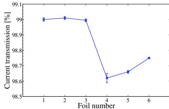
Figure 3: Current transmission between the downstream and upstream BCT for different foils (see Table 1).
