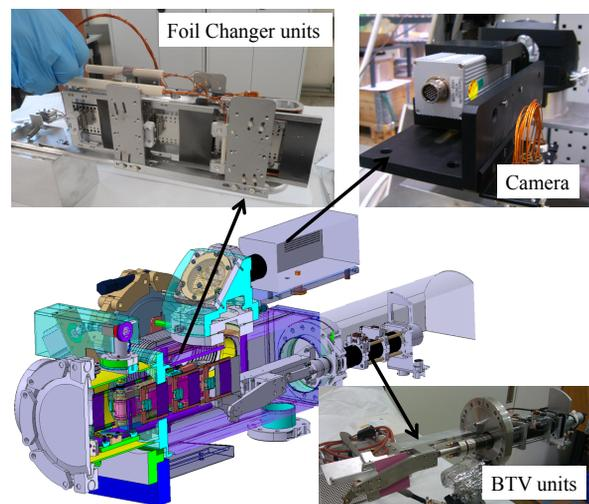
Figure 1: The stripping foil unit including the integrated BTV screen and camera.
