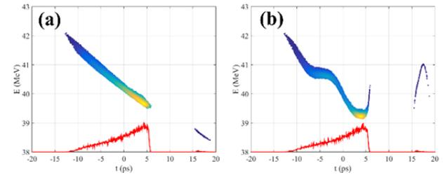
Figure 5: Longitudinal phase space before (a) and after (b) the CWFA structure. Red curves are temporal profiles.
