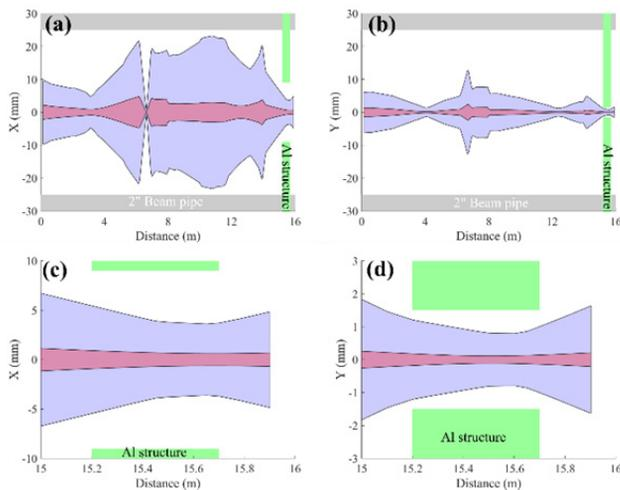
Figure 3: Horizontal (a) and vertical beam (b) envelope along the double EEX beamline. The red envelopes show the sigma for x and y, and the blue envelopes shows the full size of the beam for x and y. (c) and (d) shows the beam envelopes near the structure.
