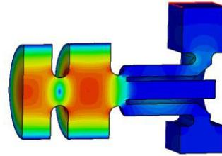
Figure 8: pi-mode electric field in full model.
