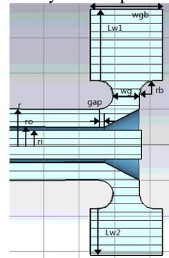
Figure 4: Cross section of coupler transformer structure.
