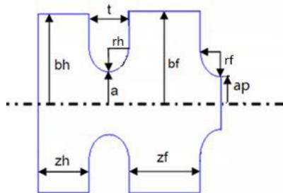
Figure 3: parameter position of gun cavity.
