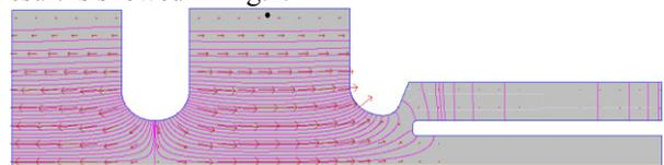
Figure 1: 2D model of the full model with pi-mode electric field in superfish.
