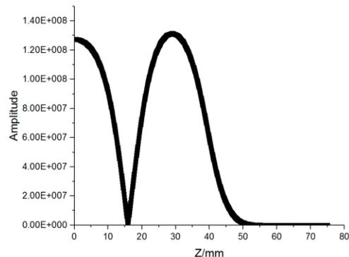
Figure 2: Ez of pi-mode along axis.
