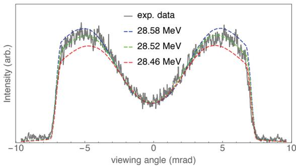
Figure 6: Effect of mean energy on lineout profile ( $\sigma_E = 0.07 \%$ ,  $\sigma_\theta = 1.8 \text{ mrad}$ ).
