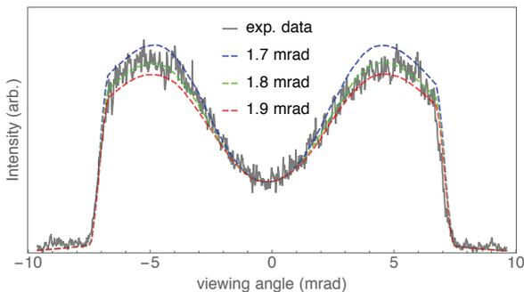
Figure 8: Effect of beam divergence on lineout profile ( $\bar{E} = 28.52 \text{ MeV}$ ,  $\sigma_E = 0.07 \%$ ).
