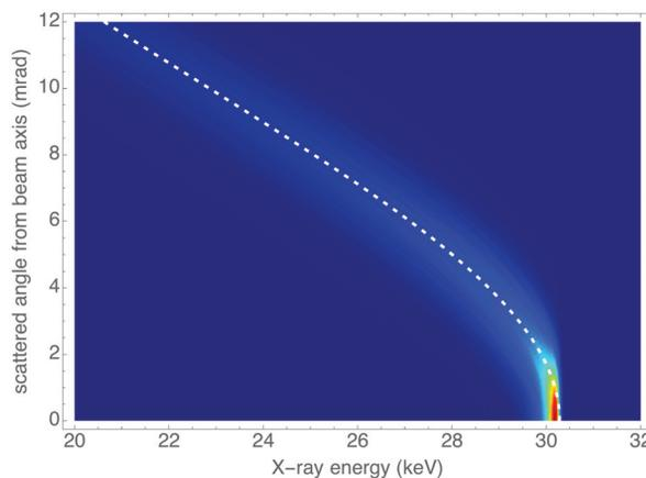
Figure 1: Energy-angle spectrum for a divergence-dominated beam ( $\sigma_\theta = 1$  mrad,  $\sigma_E = 0.06\%$ ). Dashed line corresponds to Eq. (1).
