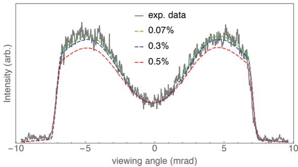
Figure 7: Effect of energy spread on lineout profile ( $\bar{E} = 28.52 \text{ MeV}$ ,  $\sigma_\theta = 1.8 \text{ mrad}$ ).
