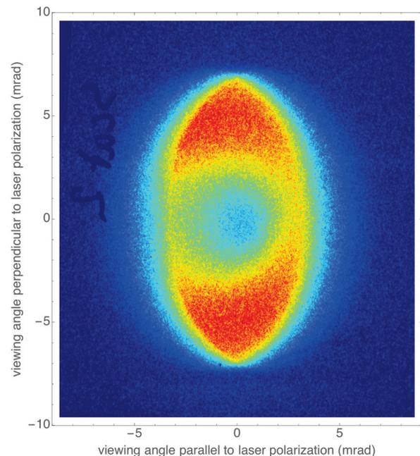
Figure 5: 30-minute integration image of Sn-filtered laser-Compton X-rays.
