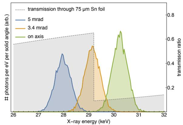
Figure 4: Local X-ray spectra at various observing angles and transmission through 75  $\mu\text{m}$  thick Sn foil.
