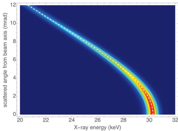
Figure 2: Energy-angle spectrum for an energy spread-dominated beam ( $\sigma_\theta = 0.2$  mrad,  $\sigma_E = 0.5\%$ ).
