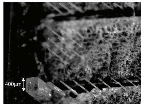
Figure 4: A photograph of the partially developed PMMA resist. The observation angle is approximately 30 degrees such that the depth of the structures is visible.
