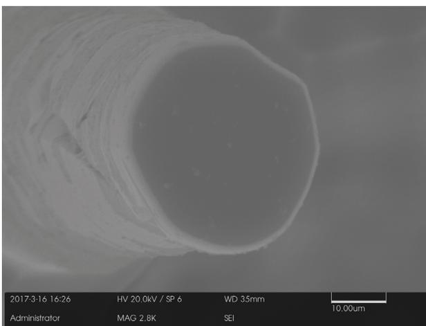
Figure 6: An SEM image of the partially developed PMMA resist as viewed at an angle of 3 degrees.
