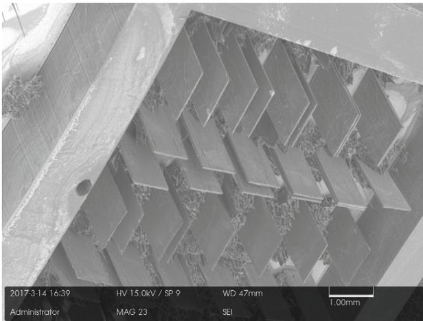
Figure 5: An SEM image of the partially developed PMMA resist as viewed at an angle of 60 degrees.
