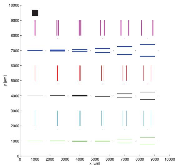
Figure 2: Screen design for interferometry and direct imaging using slits and square apertures.
