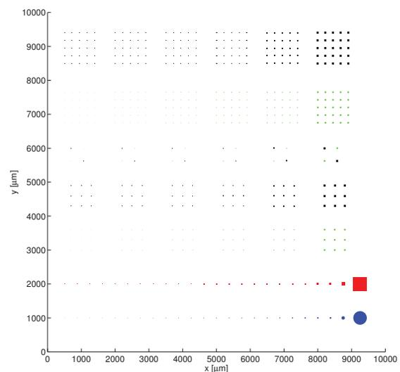
Figure 1: Screen design for direct imaging of the electron beam using circular or square apertures. The aperture sizes range from 10 μm to 400 μm.
