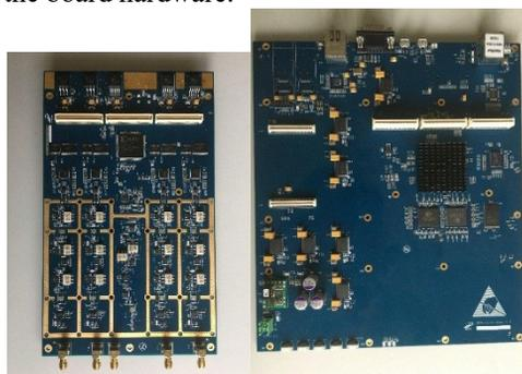
Figure 6: RF board (left) and Digital board (right) hardware.
