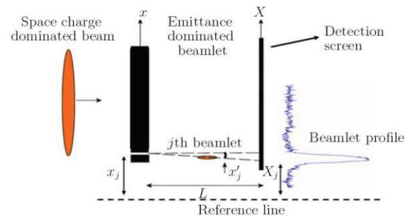
Figure 1: Slit-based emittance measurement scheme. Taken from [6].
