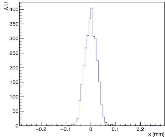
Figure 4: Typical beamlet profile at the detection screen.
