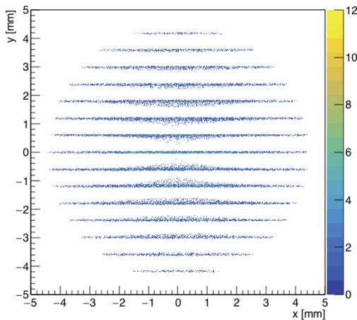
Figure 3: Beamlet image produced by a 15 x 50 μm multi-slit with 600 μm spacing as seen at the detection screen.
