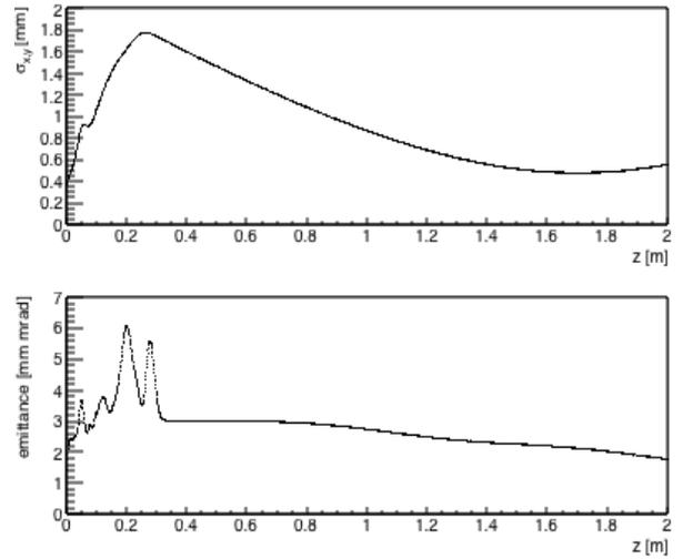
Figure 2: Envelopes and emittance as a function of the longitudinal beam position.
