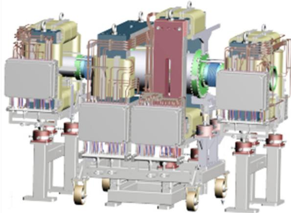
Figure 1: Ionization Profile Monitor with window frame magnets.
