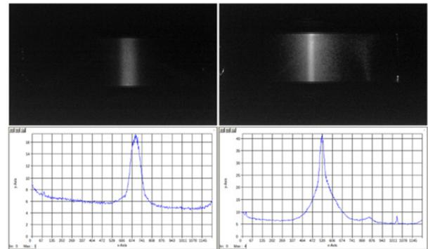
Figure 2: Example IPM data: raw ccd images (top), hor. (bottom, left), vertical profile projection (bottom right).
