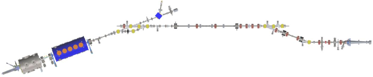
Figure 2: The layout of the low energy part of bERLinPro: the diagnostic line in straight continuation of the gun with the spectrometer arm, and the so called ‘Banana’ with quadrupoles replacing the linac module and the high power beam dump.
