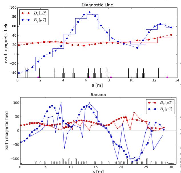
Figure 1: Earth magnetic field ( $B_x$ : red dots,  $B_y$ : blue dots) measured along the future electron path. Top: Diagnostic line with approximating step functions; Bottom: Banana with control measurement after magnet installation.
