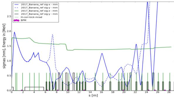
Figure 5: Beam size (x-blue; y-dashed, z-green) at 6.7 MeV and 77 pC; magnets (black), correctors (green) and BPMs (magenta) in the Banana; beyond 24 m the beam is widened for the dump.
