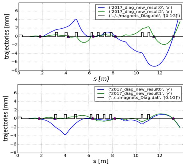
Figure 6: Diagnostic line, green, top: horizontal plane; bottom: vertical plane, correction with 2 and 1 virtual BPMs, respectively (triangles). Blue: regular correction.
