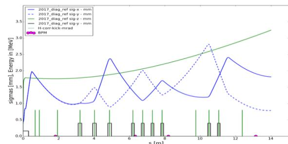
Figure 4: Beam size (x-blue; y-dashed, z-green) at 2.7 MeV and 77 pC; quadrupoles (black), correctors (green) and BPMs (magenta) in the Diagnostic line.
