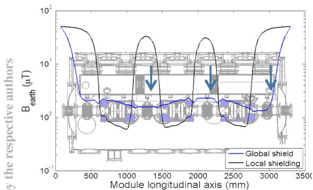
Figure 3: Simulations of the penetration of a 50  $\mu\text{T}$  outer field onto the axis of the booster module with global (blue) and local (black) magnetic shielding. The arrows indicate the corrector positions.
