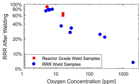
Figure 3: The relative RRR measured after TIG welds performed in the glove box with different ambient oxygen concentrations, compared to the pre-weld RRR.
