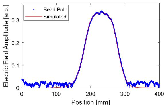
Figure 5: Bead pull measurement of the operating mode showing good agreement to the simulated field profile.
