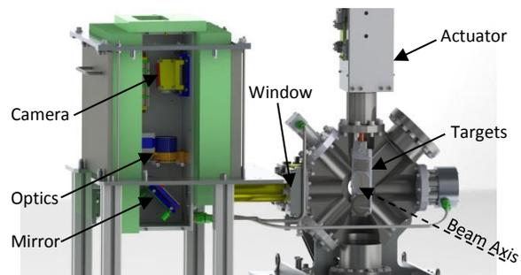
Figure 1: The view screen system installed on the beamline showing the target ladder and imaging system.
