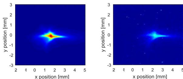
Figure 3: The beam profile from the P46 scintillation target (left) and PG OTR foil (right) imaged from the same view screen system.
