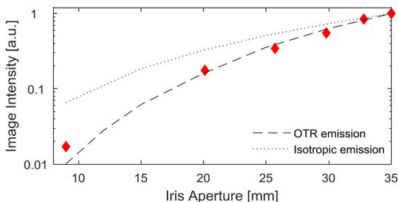
Figure 5: OTR image intensity (♦) with changing iris aperture compared to the expected intensity from the OTR emission distribution or isotropic emission.
