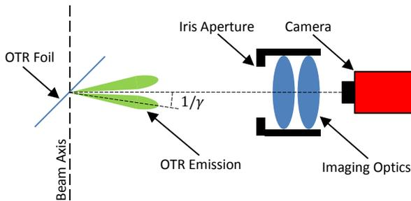
Figure 4: A schematic of the OTR emission distribution relative to the imaging optics (not to scale).
