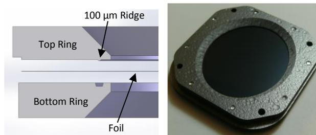
Figure 2: The ridge and groove mounting assembly, showing a mounted PG foil on the right. The mounting rings are flat and smooth, despite the appearance.
