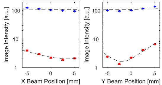
Figure 6: OTR image intensity with the beam scanned in horizontal (left) and vertical (right) directions across the screen, with the iris open (♦), and closed (■). The dashed lines show the comparison to expected image intensity.
