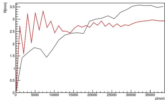
Figure 2: Beam radius along the channel before (black curve) and after (red curve) the GA optimization.
