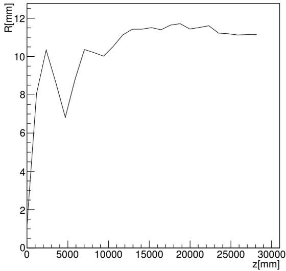
Figure 4: Beam radius along the channel. The source beam has an RMS angular spread of 100 mrad and momentum spread of 5 MeV/c.
