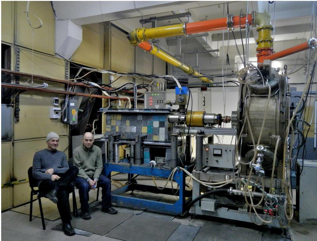
Figure 8: New electron RF gun for Novosibirsk ERL.
