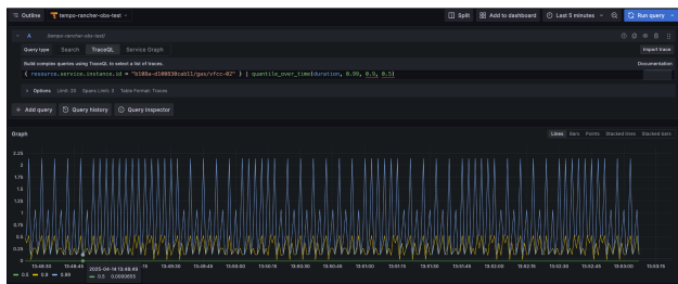
Figure 11: Example of the time duration quantiles for spans accessing the BrooksMFC Tango device. The fastest 50% of calls are under 1 ms, the fastest 90% of calls are under 0.5 s, and the 99% quantile shows the slowest calls take between 1 s and 2 s.
