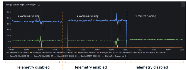
Figure 13: CPU usage trend for a single host running multiple Tango camera device servers, with up to two capturing images. Telemetry was initially disabled, then enabled for four hours, and then disabled again.
