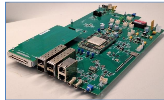
Carrier board prototype design by SOLEIL; populated with enclustra SOM and D-tacq ACQ427
