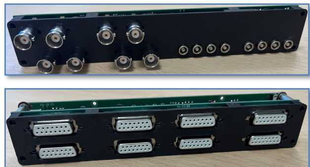
Figure 7: On top the DIO board prototype and below the Encoder board prototype.
