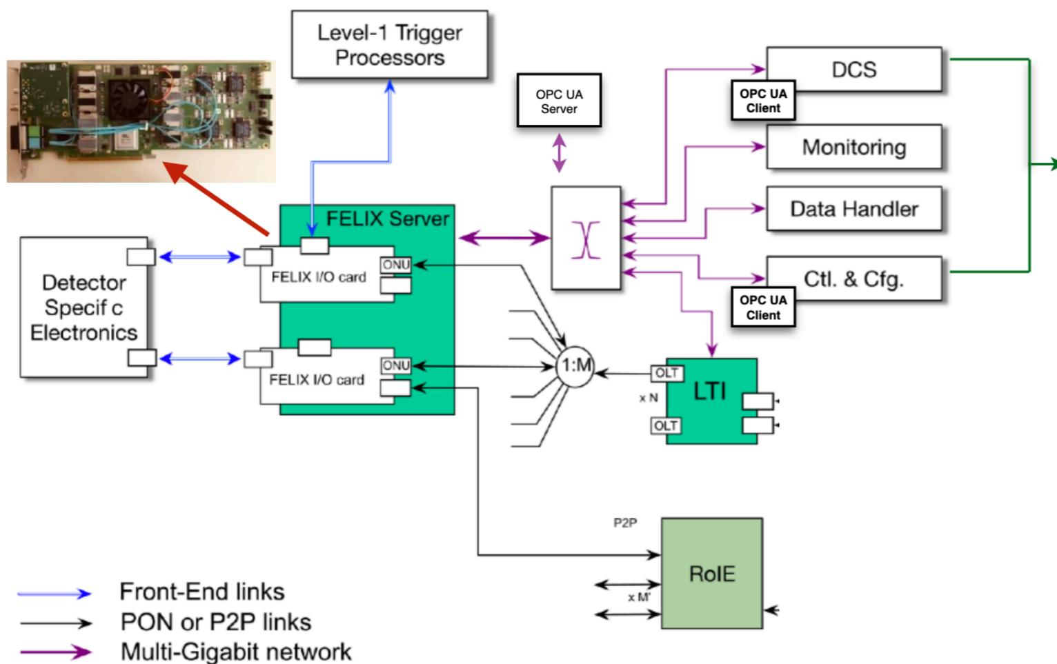
▶ DCS, Calibration & Configuration share the common path to the detector electronics (through GBT-SCA) and the SCA OPC UA Server which developed by ATLAS Central DCS
