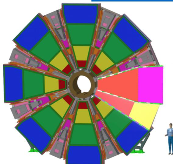
The NSW will provide high precision muon track reconstruction and trigger information to ATLAS, at high rates, thus eliminating the issues of the present SW.
