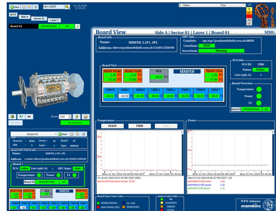
For each individual layer, a main panel has been developed, providing the user with useful information, reflecting the state and status of the detector.
