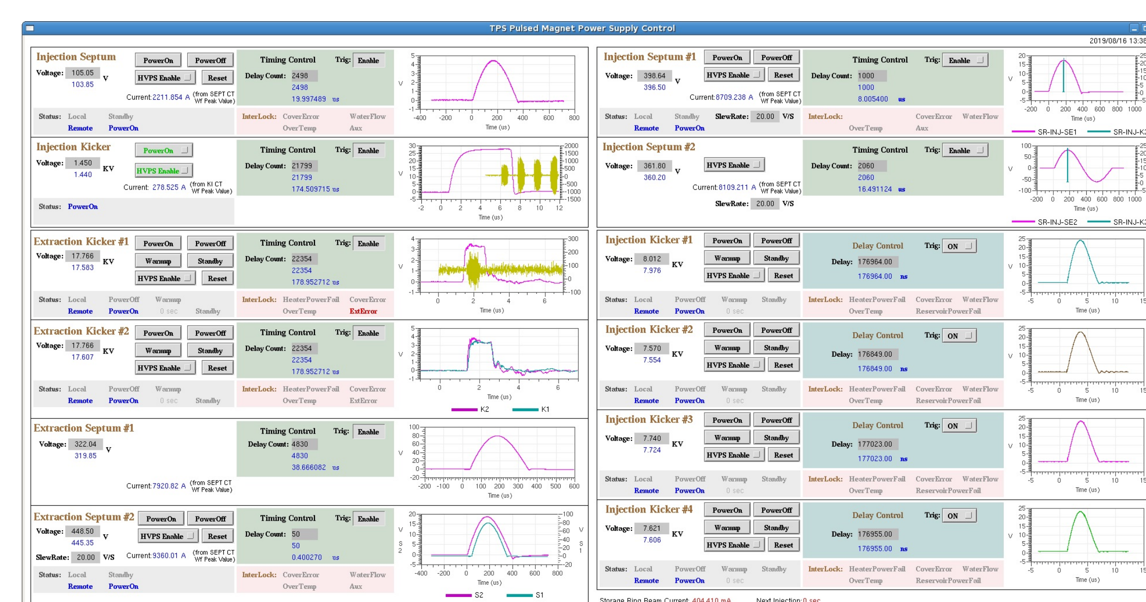
Figure 4: Several credit-card sized waveform acquisitions employed and integrated into the sub-systems of TPS: GUI of TPS pulsed magnets power supplies.
