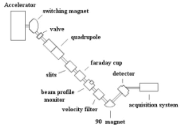
Figure 2: Isotope Separator on the 45° port.
