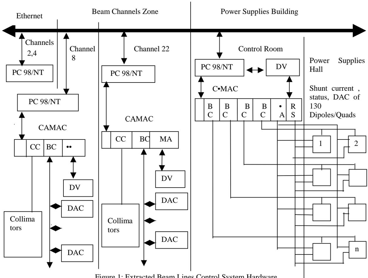
Figure 1: Extracted Beam Lines Control System Hardware.
