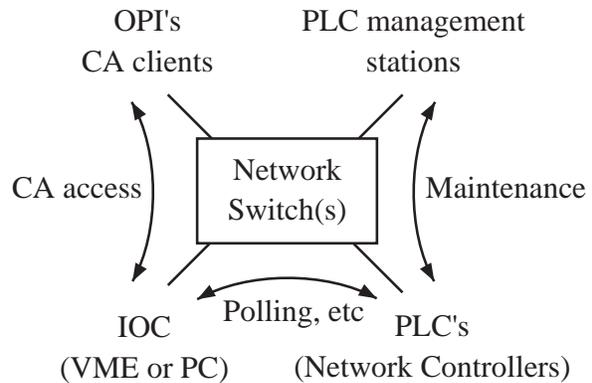
Figure 1: The same network is shared between different purposes between network controllers, EPICS IOCs, EPICS OPIs and management stations.
