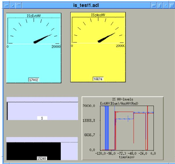
Figure 2: An example panel for testing the ion source of the linac, which utilizes the EPICS PLC records.
