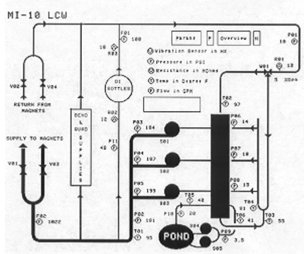
Fig. 2: Graphic View of MI-10 LCW System
