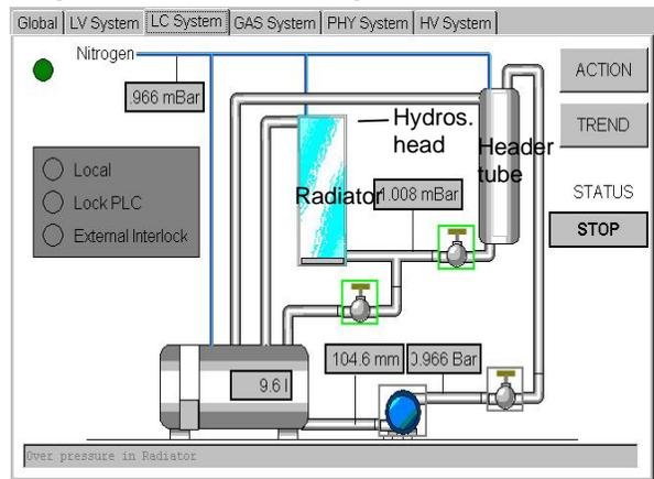
Figure 4: Schematic of the liquid circulation system
