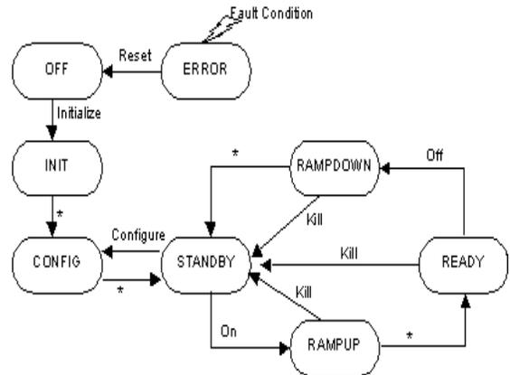
Figure 3: The bubble chart of the HV system.
