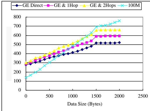
Figure 3: Measured latency of the GE and FE.
