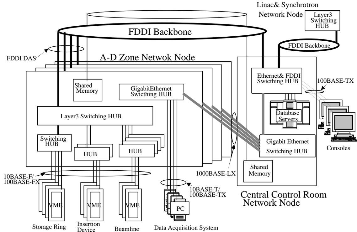
Figure 1: Schematic view of the SPring-8 network.
